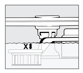
The water level is correct when dimension "X" is at least 1/8 "(4 mm).
